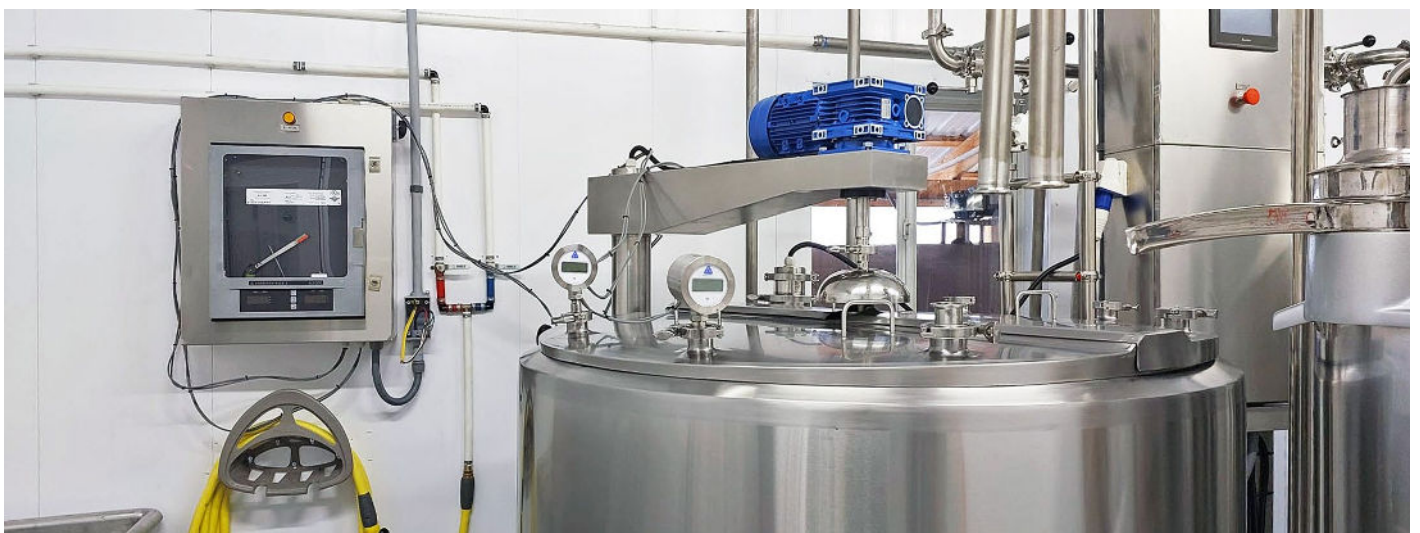
A VAT batch pasteurizer equipped with temperature sensors for the product and air space, as well as a recording system in accordance with PMO specifications (M-b certified)
